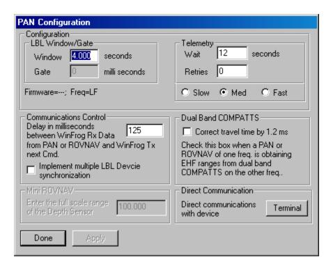
The Slow, Medium and Fast radio buttons set the telemetry baud rate through the water. See PAN manual for details on the BN and BF and BS commands. When the ROVNAV device is first selected for use it automatically send the commands mentioned above to initialize the RovNav.
